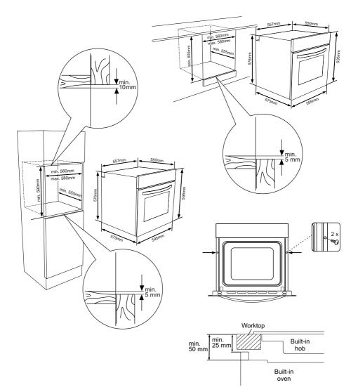
Insert the oven into the cabinet by pushing it If the oven is installed under a hob, the forward. Open the oven door and insert 2 screws in the holes located on the oven frame. While the product frame touches the wooden surface of cabinet, tighten the screws.
