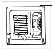
Pull the wire shelf as shown in the picture. After releasing it from clips, lift it up.
